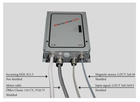
EMC glands must be used for shielded cables.
